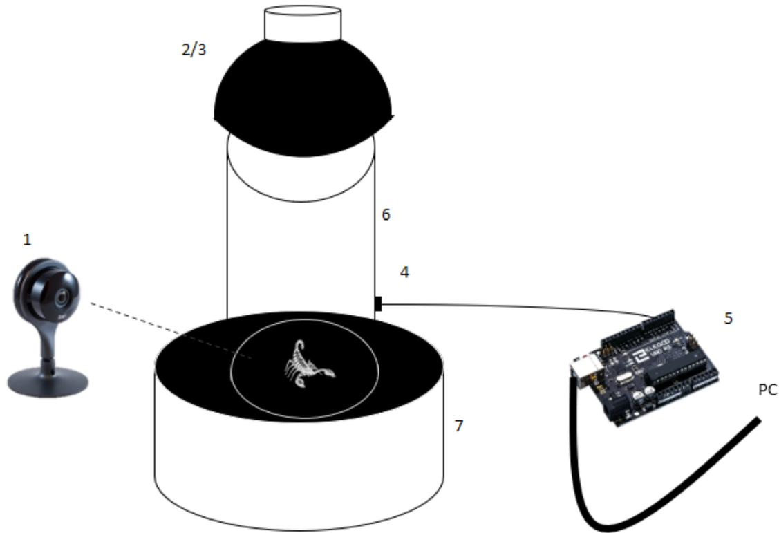
**Fig. 1:** Experimental apparatus. A Nest camera (1) recorded the experimental trials. A heat lamp (2) and the infrared ceramic heating bulb (3) heated the enclosure without producing light. A sensor (4) monitored and relayed temperature data to the microcontroller (5). The testing chamber was comprised of a clear polycarbonate tube (6); a riser (7) was added to the set up to allow the camera to better record trials.
