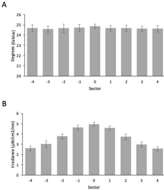
**Fig. 6:** Temperature and infrared gradients relative to the center of apparatus (pilot study). For each arena, sector 0 was oriented towards the center of the apparatus. A. Temperature values (°C) for the four testing arenas (mean +/- SE) were similar in all sectors of the arena. B. Infrared values (in irradiants; mean +/- SE) by sector for the four testing arenas were strongest near the center of the apparatus and decreased towards the exterior of the apparatus.
