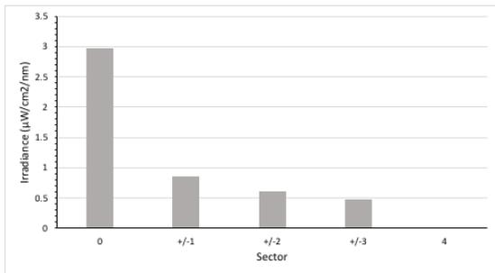
**Fig. 7:** Infrared intensity in the gradient arena. A spectrophotometer was used to measure infrared values (μW/cm<sup>2</sup>/nm) around the gradient arena to ensure a gradient existed. The control arena was calibrated to a value equivalent to sectors +/- 2 in the gradient arena.
