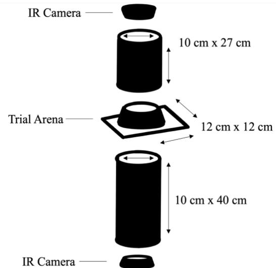
**Fig. 3:** New behavioral apparatus. Two PVC pipes were cut to create the body of the apparatus, and the removeable arenas were inserted between the two pipes. The lower IR camera provided an IR gradient to the arenas above, and the upper IR camera allowed us to visualize and track scorpion movements.
