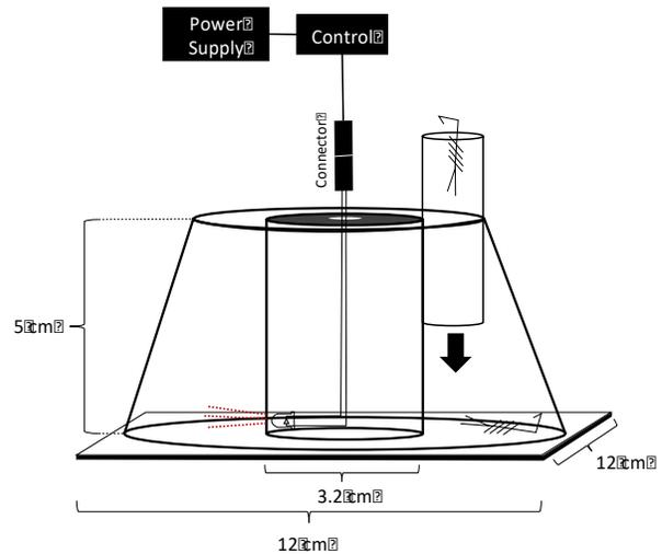
**Fig 2:** Individual behavioral arena. The arena was a plastic circular track created by a Plexiglas pipe in the middle. The center pipe contained the secured LED light that directed light across the track. The removable tube where the scorpion is held before the beginning of the experiment is pictured at the moment of releasing the scorpion from the tube.
