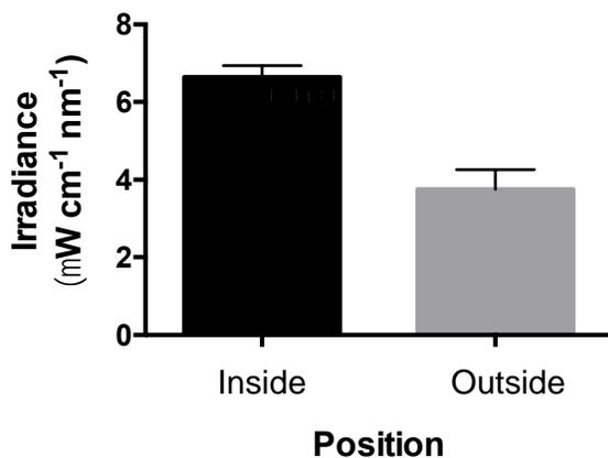
**Fig. 8:** Differences in IR levels from center to periphery of individual arenas. The irradiance on the inside of the arenas, closest to the middle of the apparatus, was larger than the irradiance on the outside of the arena.
