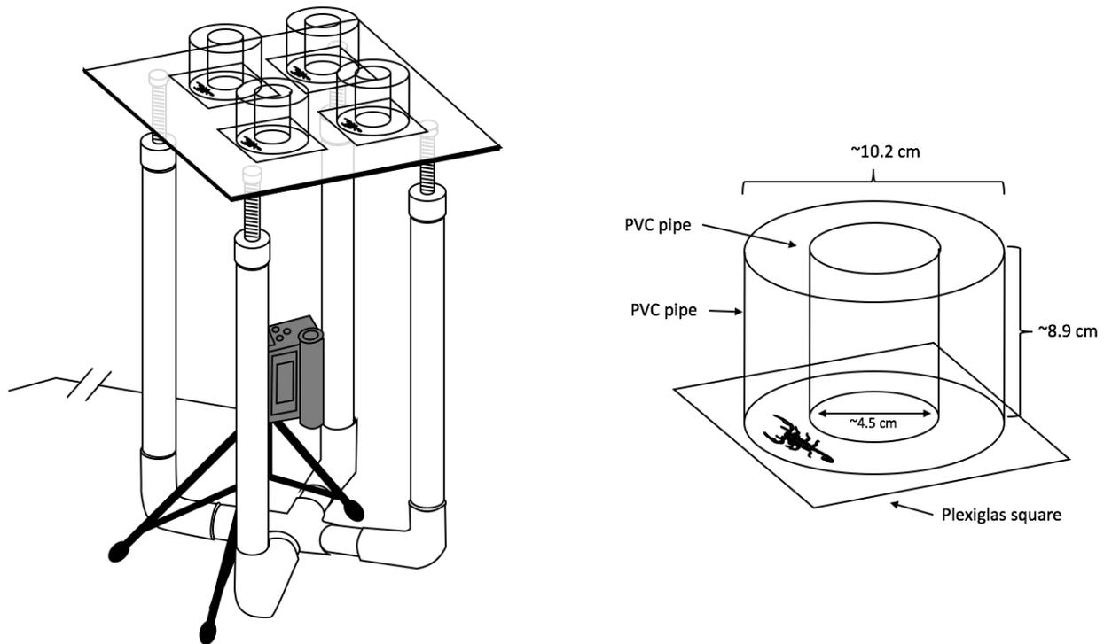
**Fig. 1:** Experimental design. Concentric PVC pipes form round tracks with open tops where scorpions with fiber optics connected to light sources can move freely. A transparent Plexiglas base provides a platform and enables video recording for later analysis. Entire apparatus was surrounded by a cardboard structure to create total darkness.
