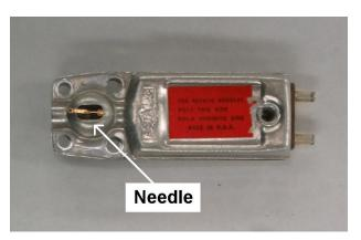
After testing, the cartridges were pried open and the transducer itself was used as the receptive element. This approach benefited from the increased surface area for receiving the waves, but suffered due to the fragility of pre-attached electrodes. Several electrodes were torn during handling.
