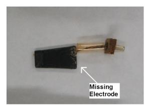
Finally, the cartridge was altered by cutting away part of one of the sides, exposing the transducer but allowing it to remain within the stable casing. This seems to maximize the performance of the receivers while protecting the electrodes.
