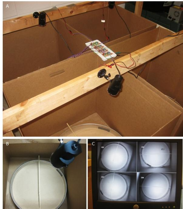
**Fig. 2:** Experimental arena set-up and recording. **A** Cameras and ultraviolet LEDs (connected to the operational amplifier unit) were mounted on a wooden frame. **B** The shadow of the dowel rod served as the artificial shelter. **C** We recorded and reviewed scorpion behavior on a security system program.
