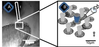
A Pictured is a field of view from a light microscope of the distal region of one tooth under mineral oil (here *Paruroctonus utahensis* female). A glass capillary tube (t) containing a chemical stimulant is introduced to the pore of the sensillum. B An electrochemically sharpened tungsten electrode is inserted at the base of a single peg sensillum to capture the neural response during chemical stimulation.
