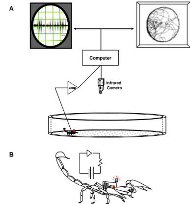
Figure 4 A *Hadruirus arizonensis* fitted with infrared diode is monitored by an infrared-sensitive video camera while an implanted electrode detects pectinal nerve activity. Computer is programmed to automatically track scorpion location within the arena (1 m diam). B Closeup of infrared diode and hearing-aid battery pack mounted on scorpion. Total weight of "backpack" is 0.6 g; useful life of battery is about 24 hr.
